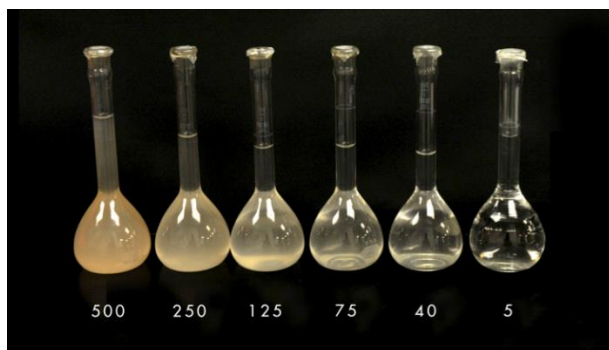
Examples of NTU readings for visual reference. Photo: MSR Water Lag Staff
